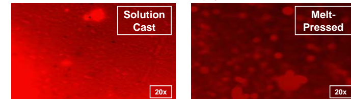
Figure: Effect of preparation on dye distribution and homogeneity: Solvent-cast and Melt-Pressed Film.
