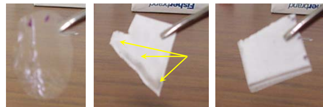
Figure: Films resulting from various prep methods: Melt-Pressed at high-temperature, high-pressure; solvent-cast film pressed at high-pressure for 1 hour (highlight of plastic deformation); solvent-cast film.
