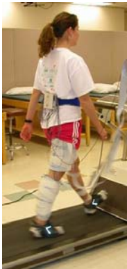
Figure: Subject donned MKI and EMG on same (day 1) and different (day 2) legs, and walked on a treadmill at 1.8, 3.0, and 6.0mph.
